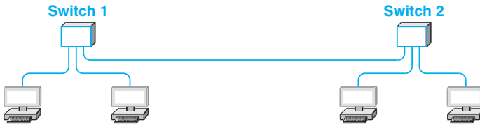
Figure 25.4 Four hosts connected by two switches.
